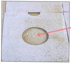
**GLUE LEAK IN** THE BASE OF JIG **THAT CAUSED GLUE STAIN**
